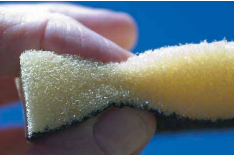
Polyimide foam is a soft, lightweight, fire-resistant material used as thermal and acoustic insulation in a variety of industries for demanding applications.
